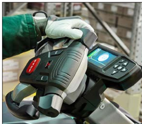
Multifunctional steering wheel with optional color display.
